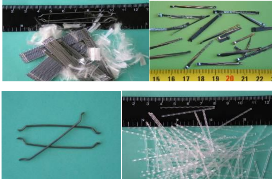
Fig.1 Top – Dra (left) and Har (right) fibres; Bottom – 50×1.00 (left) and Poliprop (right) fibres
